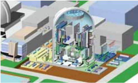
Figure 2: Cutaway of ACR-1000 showing four-quadrant design
