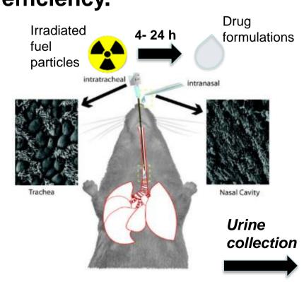
**Monitor radio-isotopes in urine:** Am/Cm, Pu238,239+240, Y-90. Radiochemical column separation and Measurements: alpha spec, ICPMS, and LSC.
