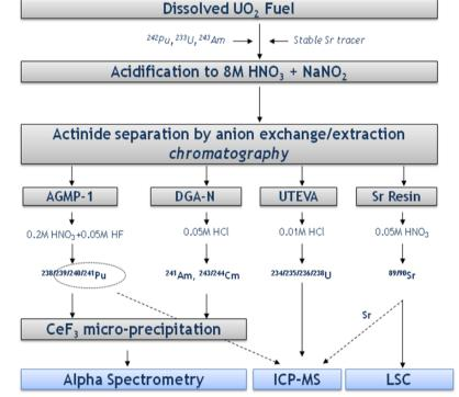
separation procedure for characterization of irradiated UO2 fuel
