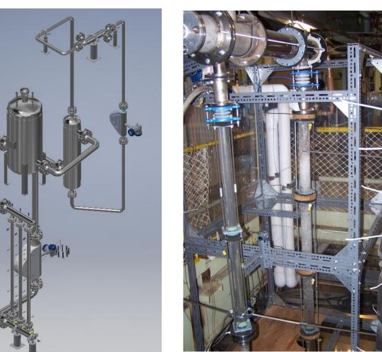
• Design and construction of coupledloop passive safety facility. Capable of studies Reactor Cavity Cooling Systems (RCCS) and Direct Reactor Auxiliary Cooling System (DRACS). Water, air, and Dowtherm-A working fluids.
