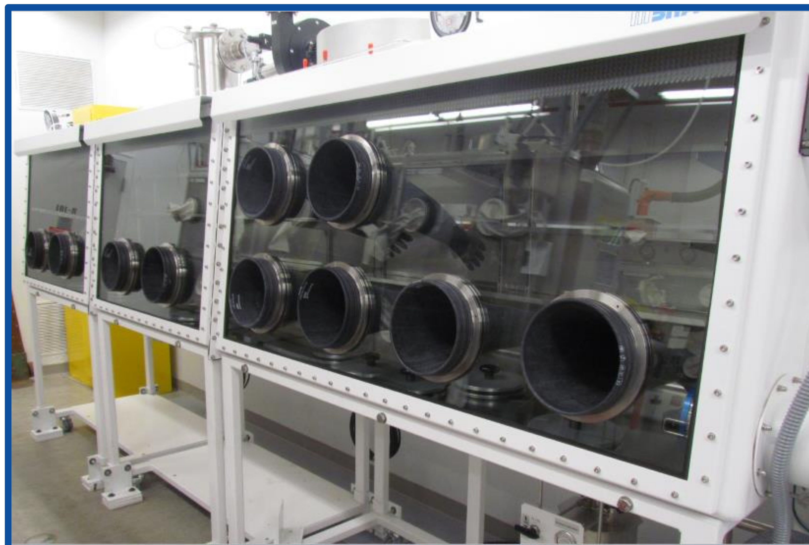
Figure: Inert atmosphere glovebox for molten salt fuel synthesis
